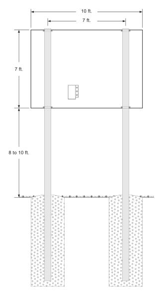
Once you have verified the positions of the posts and the size of the footings, you are ready to dig your holes, pour your concrete, and set your posts. There are several techniques for ensuring proper alignment of the posts. Typically installers will construct a temporary wooden support frame to hold each post in place while the concrete sets. Having plumb posts in the proper position is the key to a smooth mechanical installation.
